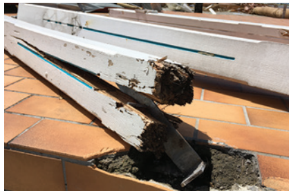
Figure 6: Posts with ripped out right-angled fixing brackets
