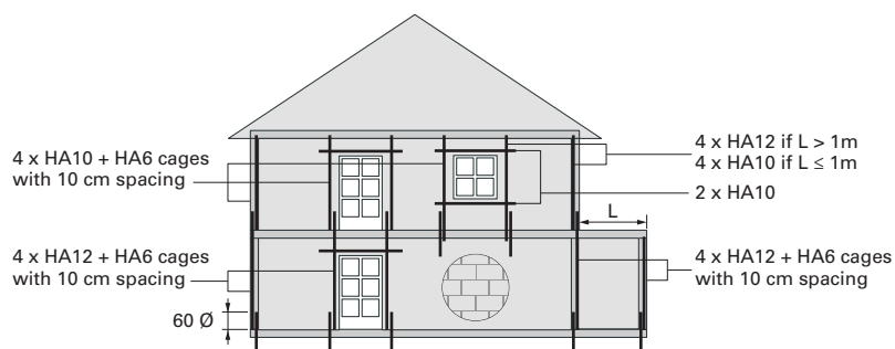
Figure 19: Example of vertical tie beam arrangement
